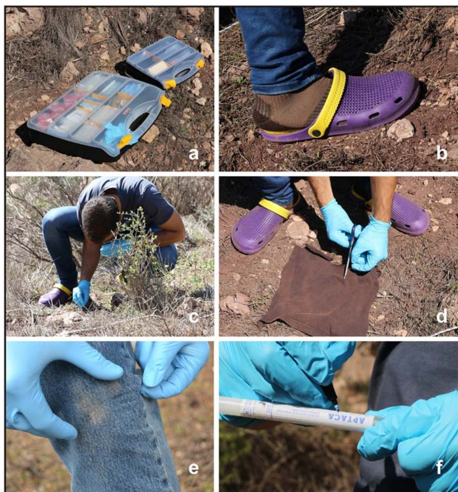
Fig. 2. Collection and sampling. (a) Equipment, material and instruments used for sampling. (b) Footwear worn during collection of samples. (c) Sampling of the soil surface. (d) Collection of fabrics samples. (e) Recovery of sediment from the surface of the trousers by using a slide with adhesive. (f) Labelling of one of the samples collected with swab.
